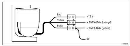
Figure 6-11: NMEA Input Connection
